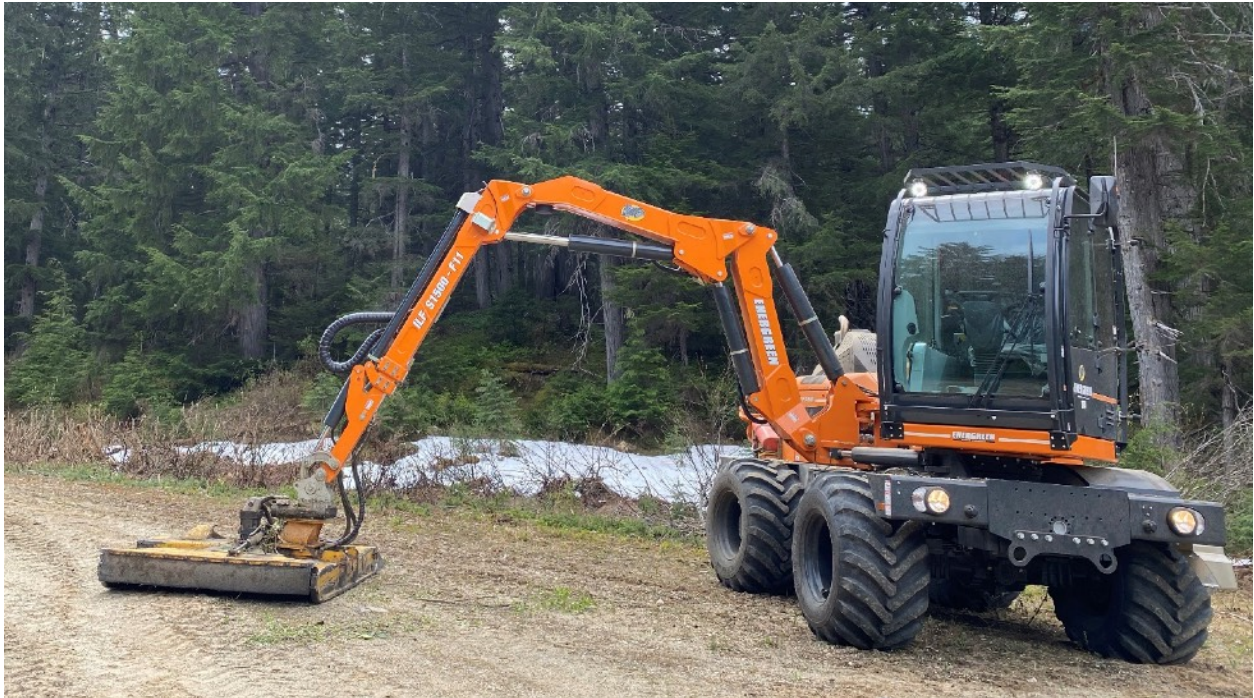
Figure 6. A self-propelled hydraulic 165 horsepower mower with a brush-cutter on an excavator arm is used for most brush-cutting work done at the present time. Photo from Graham Darragh of Valemount.
